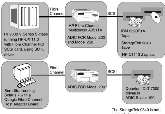
The Storage Tek 9840 is not supported as a network-attached device, only as a SCSI-attached device.
